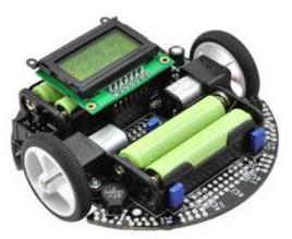
The Pololu 3pi lacks a range finding sensor; however, one can be easily soldered onto the front. The advantage of the 3pi is that it can turn in place, making it easier to program to turn around tight corners.
