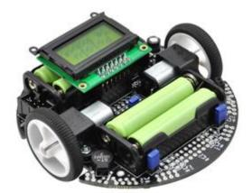
The Pololu 3pi lacks a range finding sensor; however, one can be easily soldered onto the front. The advantage of the 3pi is that it can turn in place, making it easier to program to turn around tight corners.
